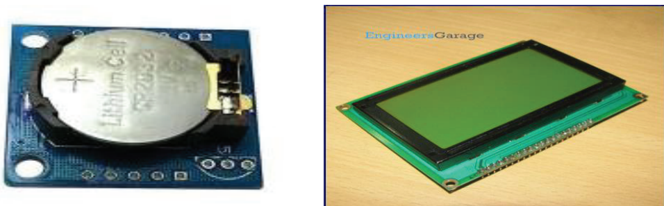
a) Real Time Clock - Real Time Clock Battery Module (DS1307).
