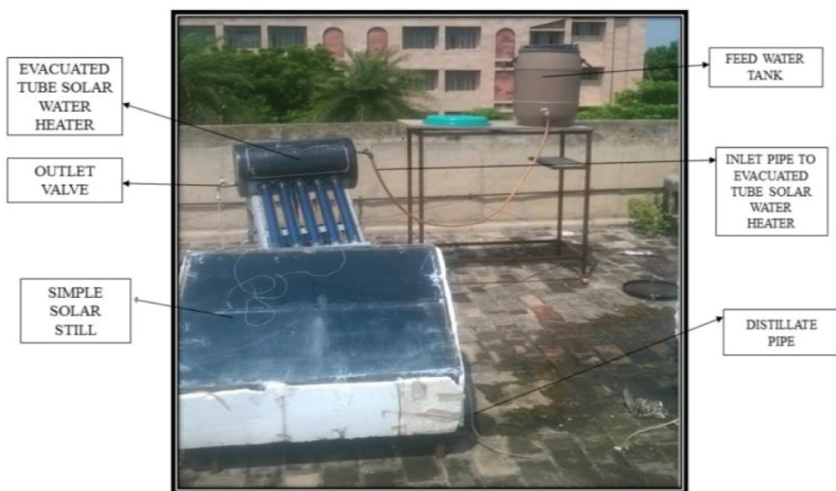
Figure 5: Direct flow through an evacuated tubular solar collector in combination with a simple solar.
